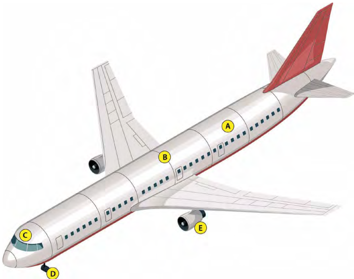
Figure 14-5: Aircraft – where asbestos might be found (non-exhaustive)
