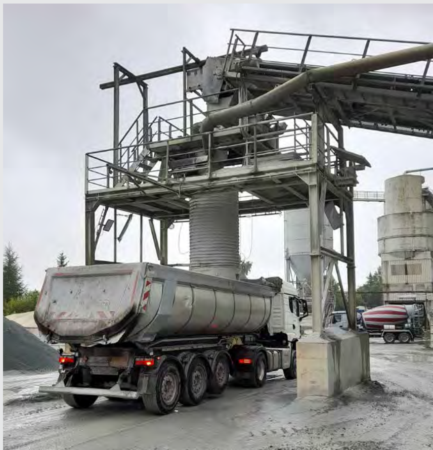
Figure 15-5: Height-adjustable truck-loading spout with dustproof skirt
